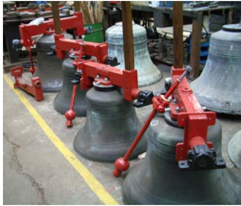
The original 3 Rudhall bells with new red headstocks and clappers and the Ringers bell which will be 5 in the ring of 6.
